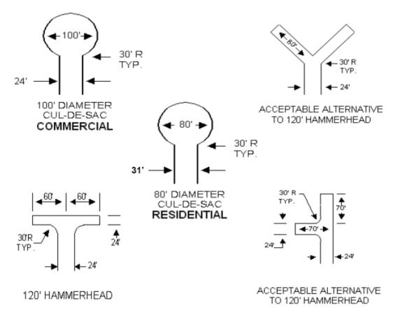
**Note:** In residential subdivisions where a proposed cul-de-sac will include an obstruction within its center, such as a planter or other impassable object, the pavement width shall measure a minimum of 100 feet.
