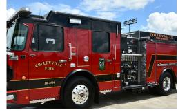
apparatus design. Engine 243 is nearly six feet shorter than other traditional engines allowing for a tighter turning radius and more maneuverability.
